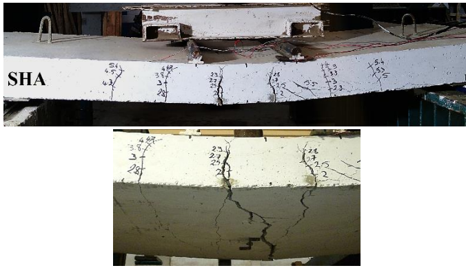
Fig. 14 Ductile flexural failure mode of hybrid slab SHA
