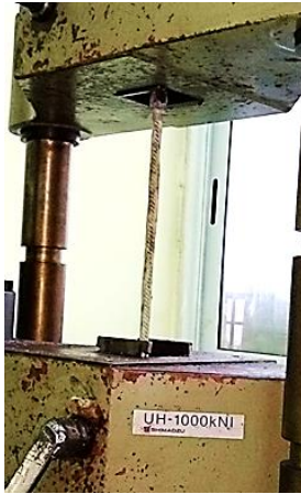
Fig. 5 Specimen and Tensile test setup
