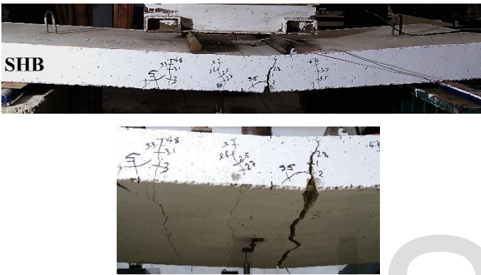
Fig. 15 Ductile flexural failure mode of hybrid slab SHB
