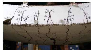
Fig. 13 Ductile flexural failure mode of hybrid slab SS
