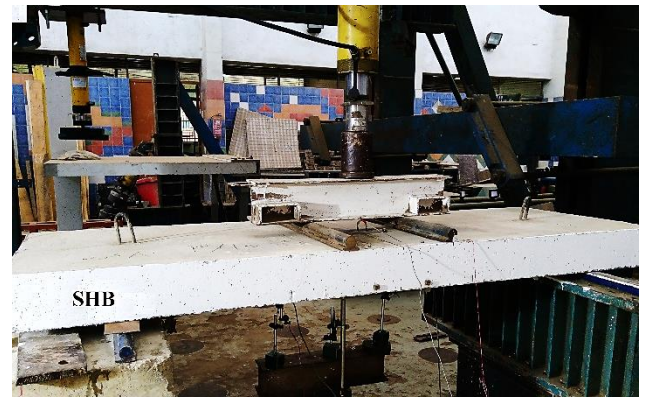
Fig. 9 Flexural test setup of concrete slabs
