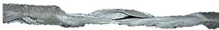
Fig. 6 HFRP with steel wires in core at failed in both glass and wires fiber
