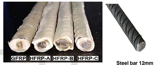
Fig. 3 Final product for development of GFRP ,HFRP Hybrid Bars and steel bar 12mm
