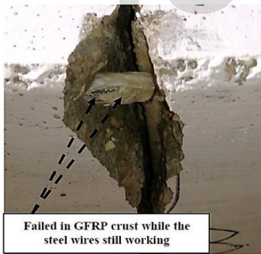
Fig. 16 The effect of hybridization in overcome the sudden rupture for type (A,B and C)
